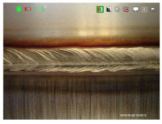
Temperature indicates on the upper left of the screen. When the testing temperature is  $20^{\circ}\text{C}\sim64^{\circ}\text{C}$ , it indicates in green color. Orange alarm when the probe temperature is  $65^{\circ}\text{C}\sim79^{\circ}\text{C}$ ; red alarm when above  $80^{\circ}\text{C}$ . For the protection of the probe and camera, the monitor will shut off automatically.
